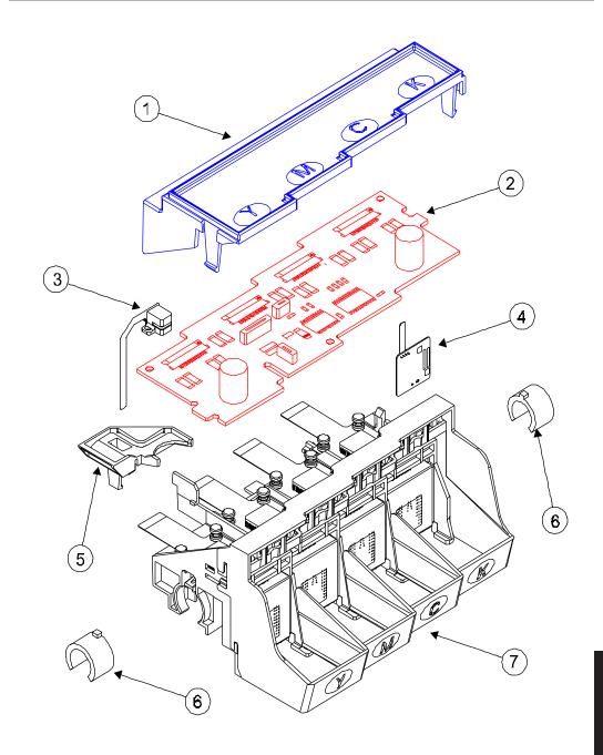
Figure 6-3. Carrier Assembly Breakdown.
